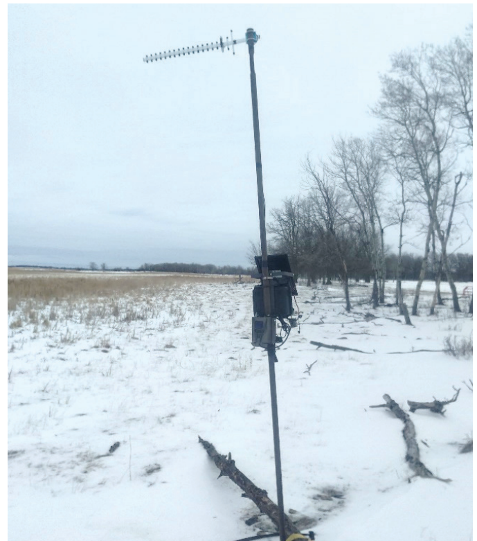
Example of fully-loaded game camera with solar power, battery, steel box and Yagi antenna.
